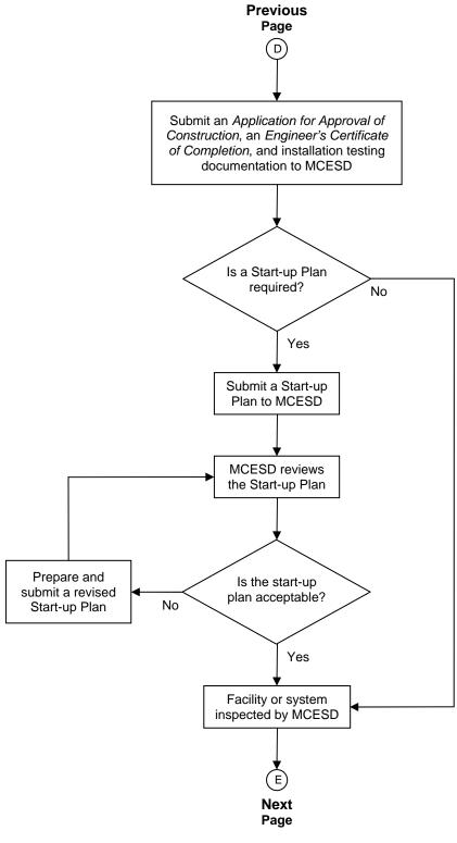
Flow Diagram of the Review and Approval Process for an Approval To Construct / Approval Of Construction for a Typical Wastewater Treatment Facility
